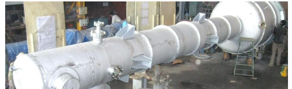
Process column in fabrication. Photo: Namindo Pty Ltd.
