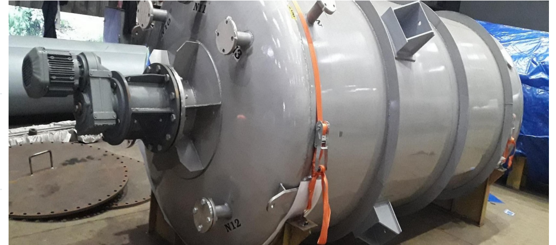
Stainless reactor vessel in fabrication. Photo: Namindo Pty Ltd.
